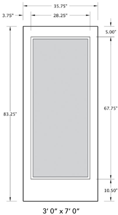
NOTE: BY REQUEST, DOOR HEIGHT COMES IN VARYING DIMENSIONS TO A MINIMUM OF 83". EXCESS WILL BE TAKEN FROM BOTTOM RAIL. ALL OTHER DIMENSIONS WILL REMAIN THE SAME.
